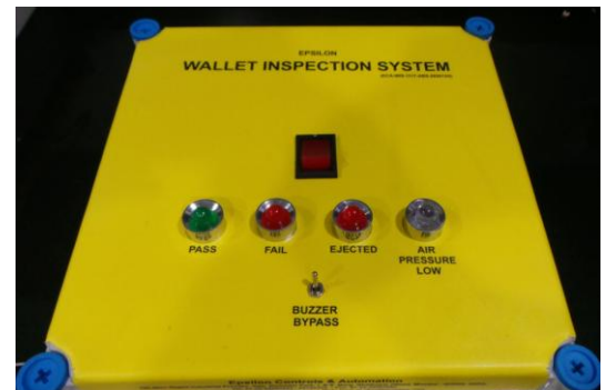
Control panel with audio visual Indication
